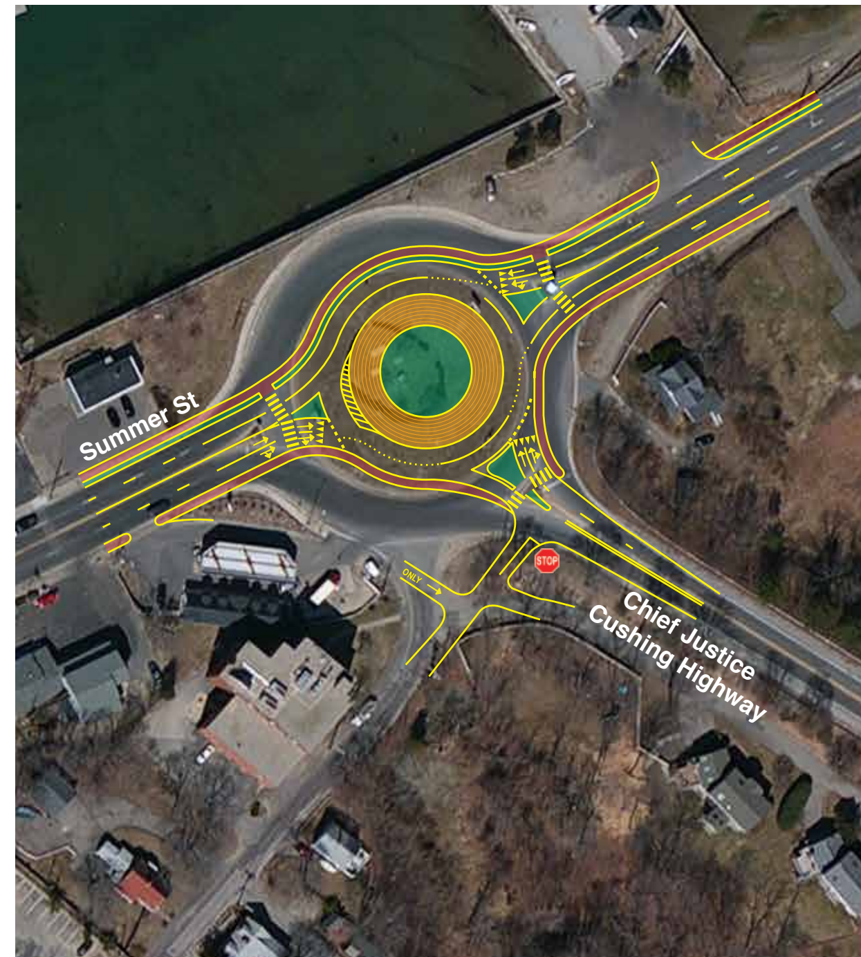
Two-Lane Modern Roundabout
