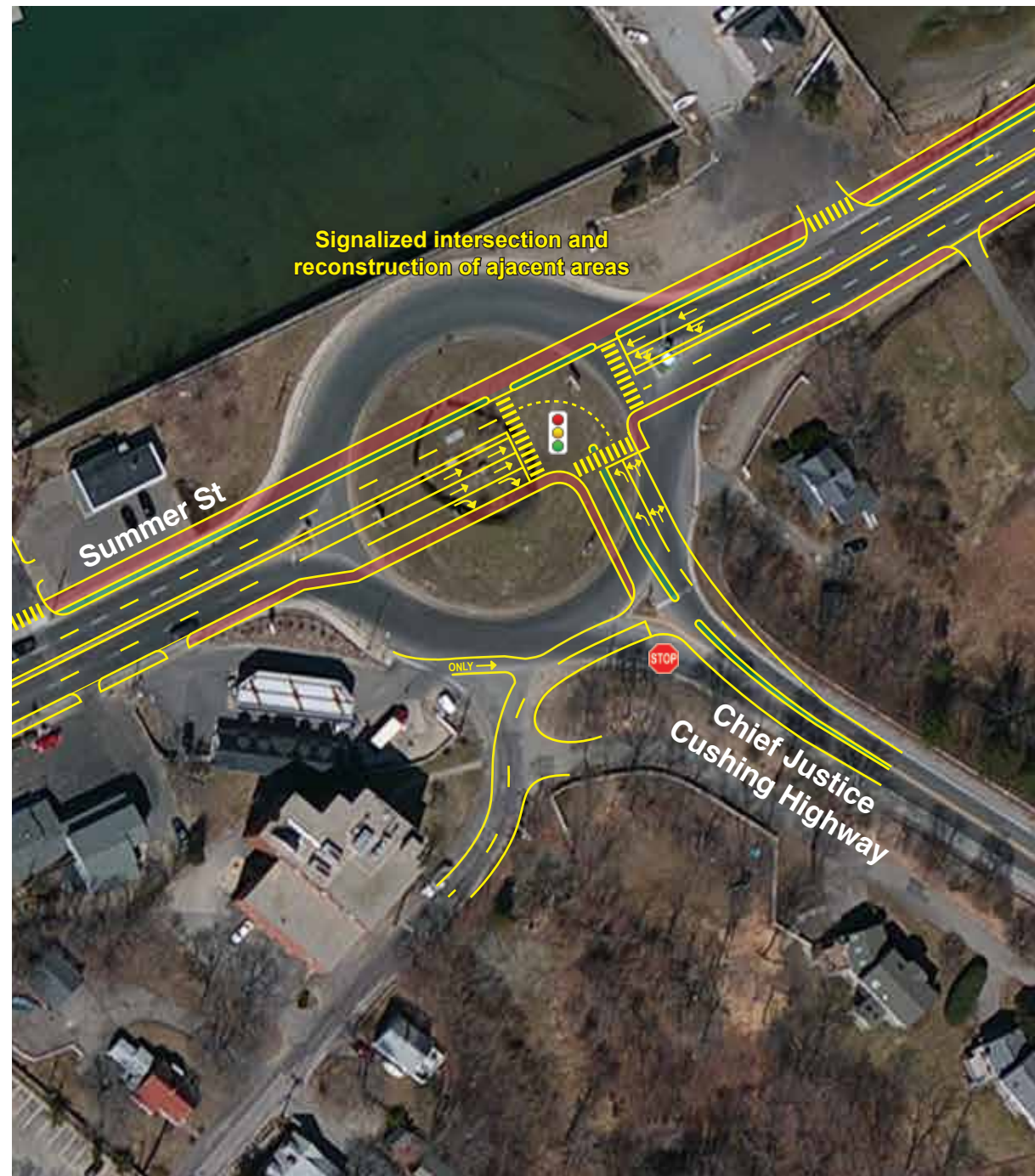
Alternative Signalized Intersection Design
